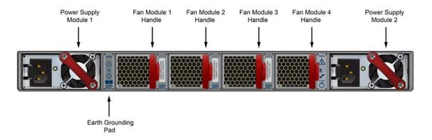
Figure D-2: Rear Panel for Models with Management Ports in the Rear
